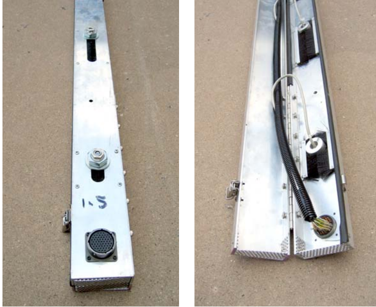
Figure 29. Sensor Side and Internal Sides of Temperature Bar.
