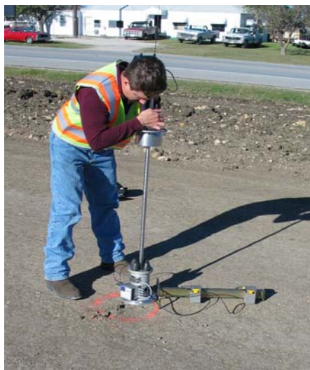
Figure 13. Portable FWD Used for Soil Stiffness Determination.
