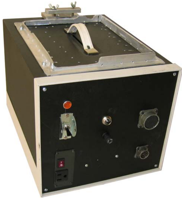
Figure 28. Master Control Box for Pave-IR.
