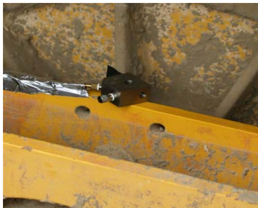
Figure 2. Accelerometer Mounted on Roller Frame.
