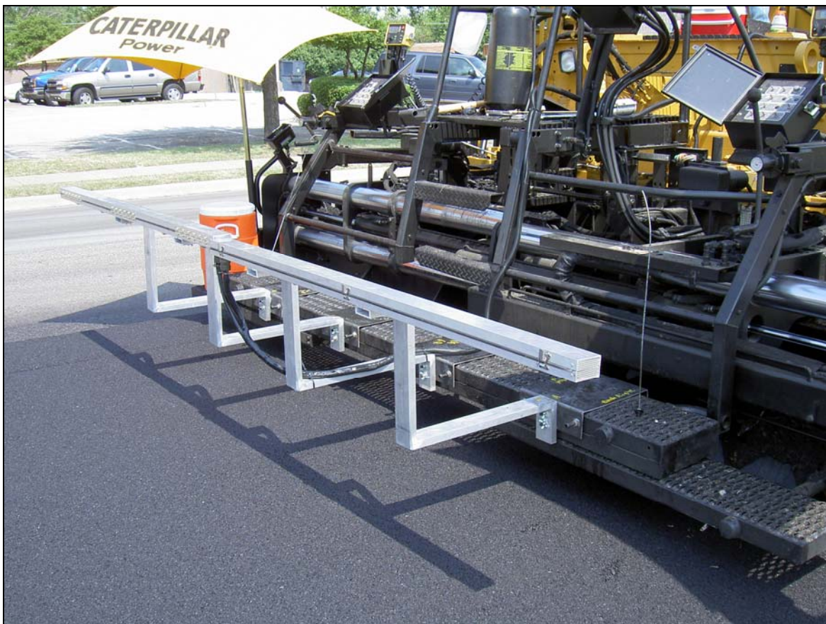
Figure 26. TTI's Current Pave-IR System Collecting Project Data.
