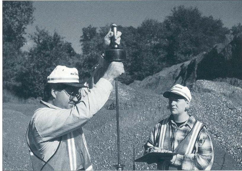
Raise the hammer to its upper limit and let it fall freely to strike the anvil. Record the penetration following each hammer drop. (Optional remote scale is shown.)
