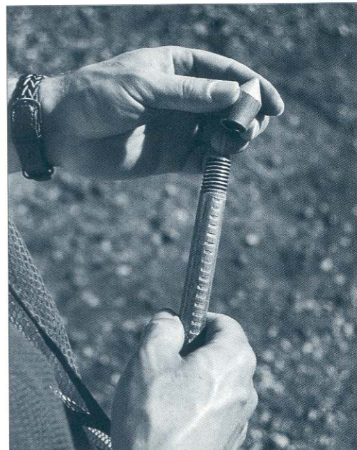
Before and after each test, examine the DCP cone tip for damage.
