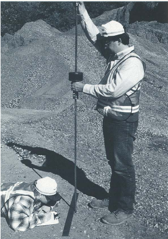
A two-person crew operates the DCP and records data manually.
