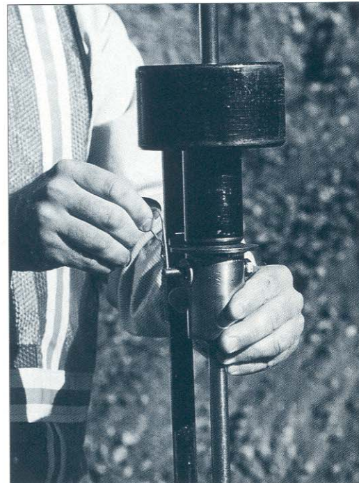
When assembling the DCP, line up connecting hole and insert connecting bolt, washer and clip pin.
