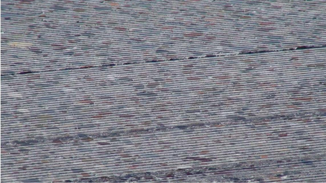
Fig 4.5 Innovative Grind with Skid Marks After Friction Testing
