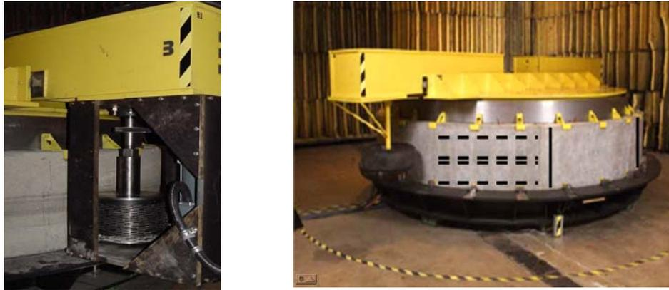
**Figure 2.1a and b Laboratory Diamond Grinder and Top Track Purdue Testing Wheel**
