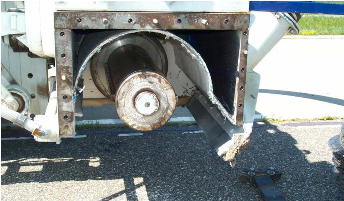
**Fig 3.2.6 Grinding Shaft before assemblage of Cutters and spacers**
