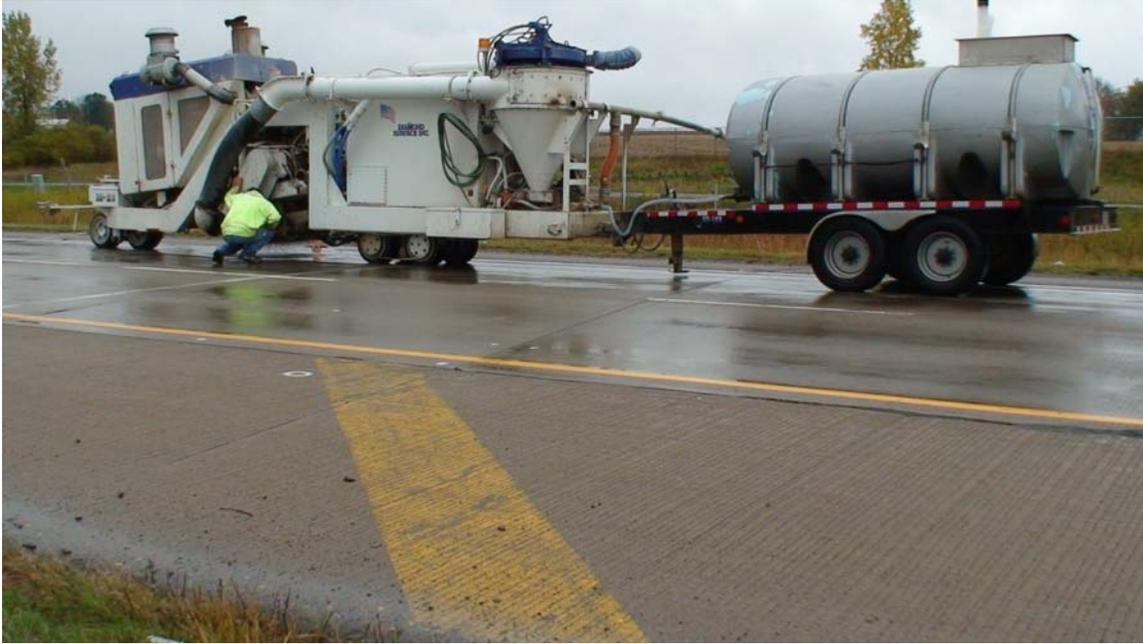
Fig 4.1 DSI Diamond Grinding equipment complete with cutter and articulated water truck
