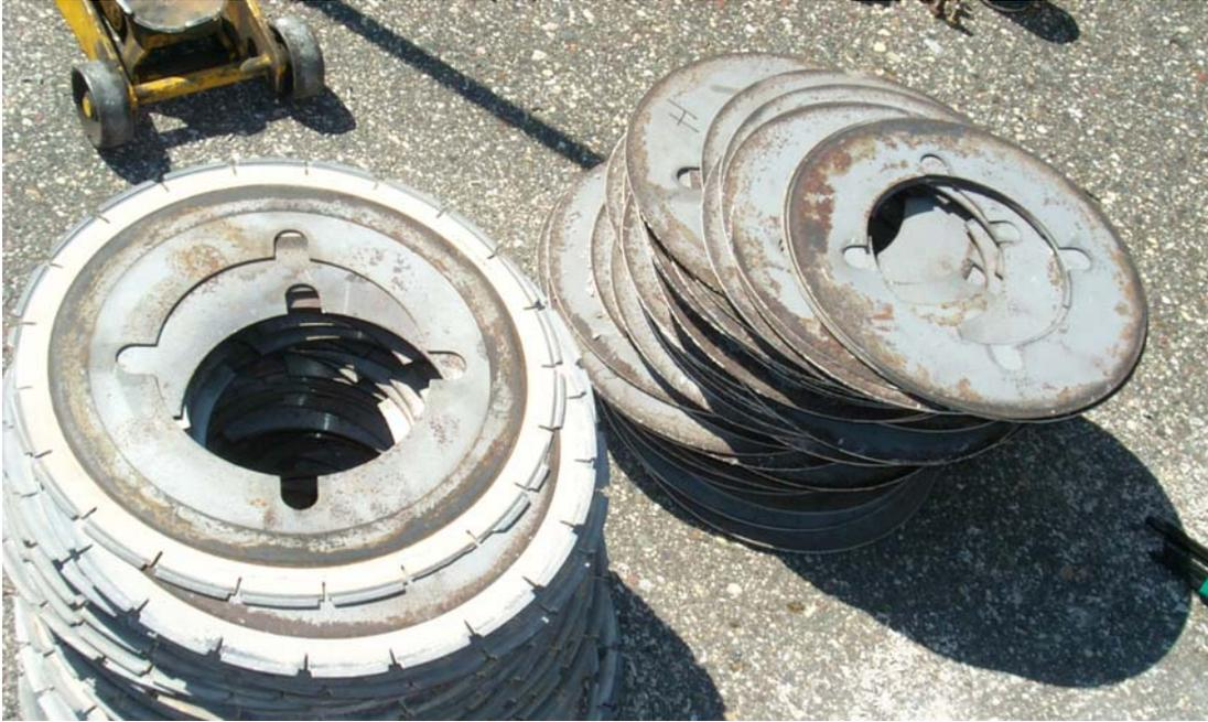
**Fig 3.2 .5 Grinding Head and Spacers**
