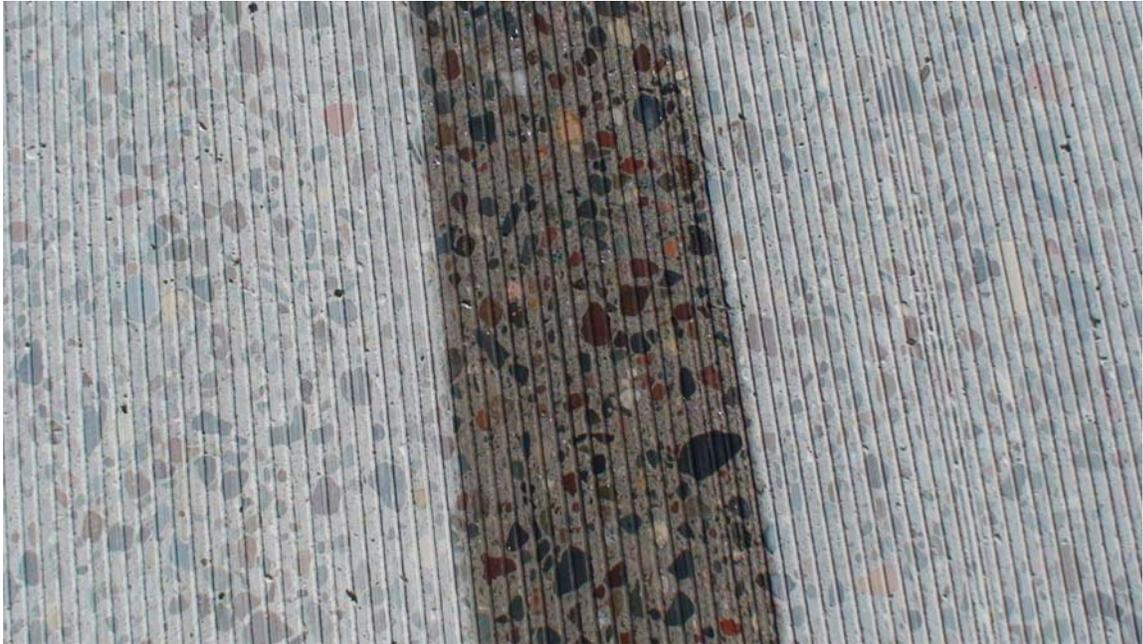
Fig 4.6 Wet Tracks on Innovative Grind After Friction Testing
