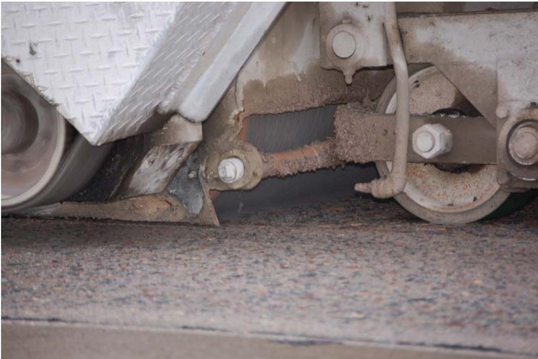
**Fig 4.10 Close-up view of the Diamond Cutter**
