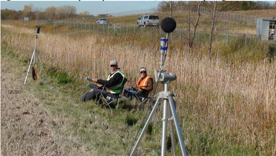
Fig 4.8 Statistical-Pass-By Showing Radar Measuring Speed Microphone and Weather Station Near cell 8
