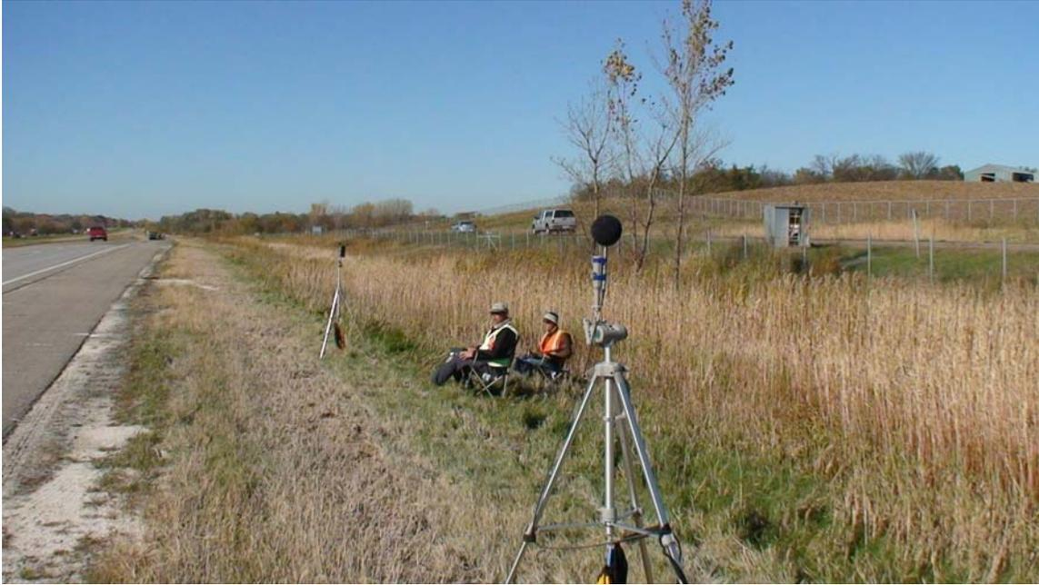
Fig 4.7 Statistical-Pass-By Set-Up Beside Cell 7 (Measurement by Illingworth and Rodkin)
