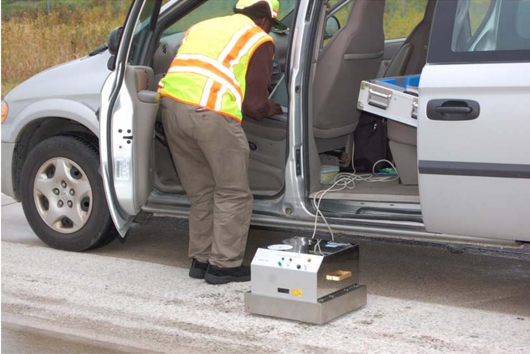
**Fig 4.9 ASTM E 2157-01 Circular Track Meter Texture Testing on cell 8**
