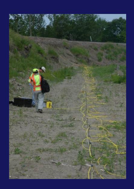
Two 8-channel resistivity/IP meters (AGI SuperSting R8/IP)
