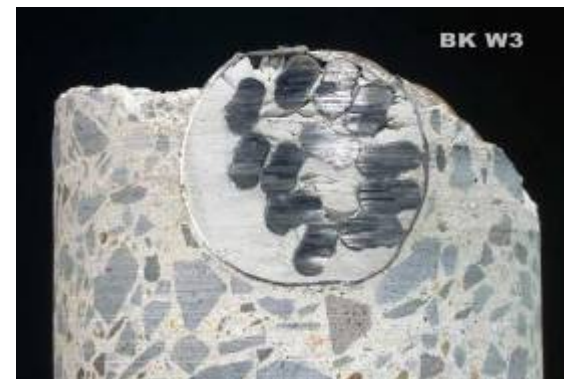
Box girder wall (longitudinal tendon ducts)
