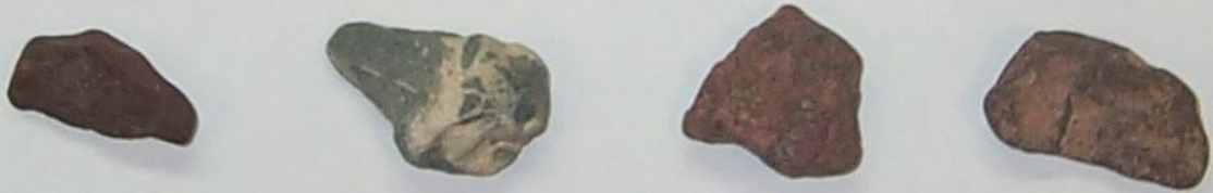
NON CRUSHED PARTICLES – ROUND EDGES, SMOOTH SURFACES
