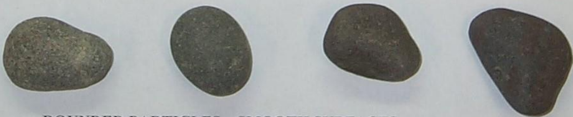
ROUNDED PARTICLES – SMOOTH SURFACES
