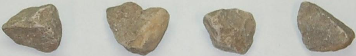
CRUSHED PARTICLES – BLUNT EDGES, ROUGH SURFACES
