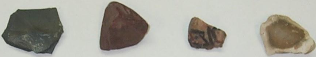
CRUSHED PARTICLES – SHARP EDGES, SMOOTH SURFACES
