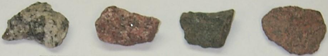
CRUSHED PARTICLES – SHARP EDGES, ROUGH SURFACES
