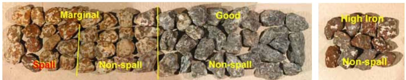
Figure 2 – Full range weathered troctolitic aggregate found in area pits from highly weathered/alterated (left) to fresh (right). Also found in the pits is a metallic looking, “high iron” variety which is not considered spall (far right).
