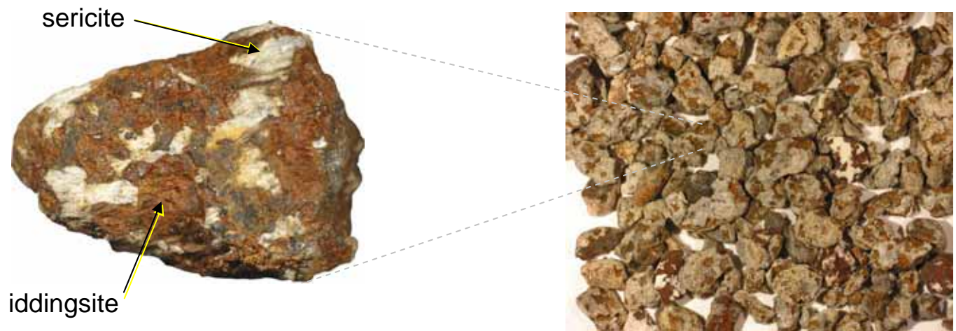
Figure 1 – 3/8-inch pile of marginal quality aggregate (right), close-up of aggregate (left)
