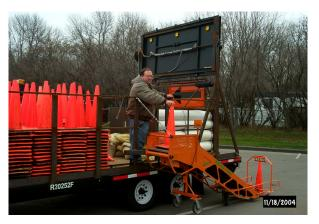
**Background:** Setting and picking up cones and other traffic control devices is one of the most dangerous jobs at Mn/DOT. When setting up a long traffic lane closer it could greatly reduce this risk if a machine could accomplish this effort.
