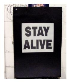
**Background:** Many new ideas in safety lighting are introduced each year. Eletroluminesense technology has been applied to Stay Back Stay Alive signs and lighted mud flaps. These will be mounted low to the ground to increase visibility of Mn/DOT trucks during plowing operations. Many times snow is lifted up when plowing resulting in snow clouds. The lighted mud flaps hopefully will allow approaching motorists an increased view of the truck under these adverse conditions.
