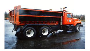
**Background:** The standard steel truck bodies require maintenance in painting, rust and dent repair, and also because of the type of rock in this area they become dented. This does not permit materials to slide out freely when dumping and especially during sanding operations.
