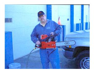
**Background:** Cutting concrete can be difficult when in confined areas. Older type concrete saws are cumbersome and awkward. When a large hole is needed one must cut beyond the edge to allow for a deep enough cut which in turn can create structural problems.
