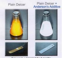
Test panels submerged for 3 months.
