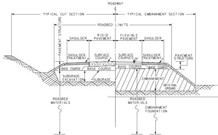
Figure 1: Typical Roadway Cross Section (Rural Section Shown)
