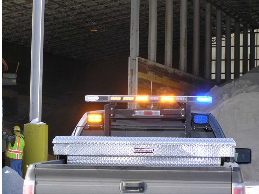
Maintenance Supervisor or Superintendent Vehicle/Area Wide Debris Patrol (Amber blue with amber blue lowers—less than 10% blue).
