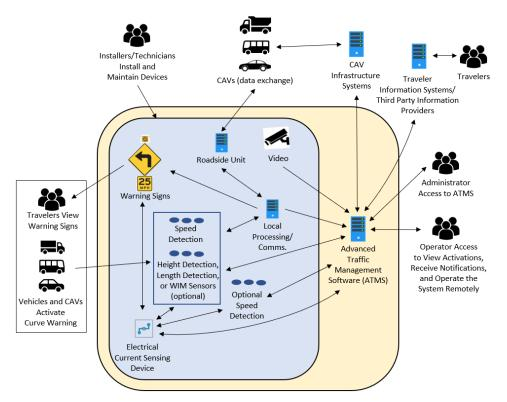
Figure 2: Illustration of Dynamic Curve Warning System Connected to ATMS - Components and Related Systems/Users
