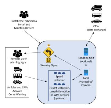
Figure 1: Illustration of Stand-Alone Dynamic Curve Warning System - Components and Related Systems/Users
