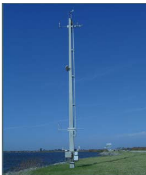
Figure 3 ESS Above Ground Sensor
