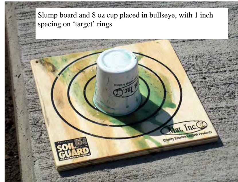
Free water slump moved more than 1 inch in 1 minute. More mixing time is required
