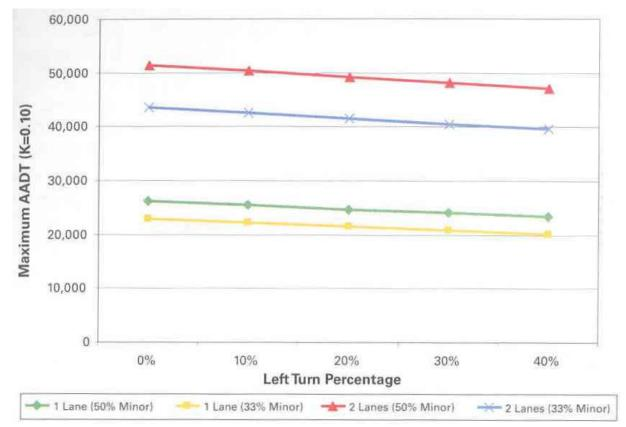
Exhibit 10: Capacity of single- and double-lane roundabouts. (source: Roundabouts: An Informational Guide, FHWA)
