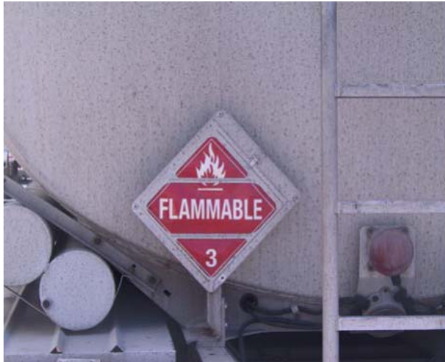
Front & Rear Placarded Flammable (No ID Numbers)
