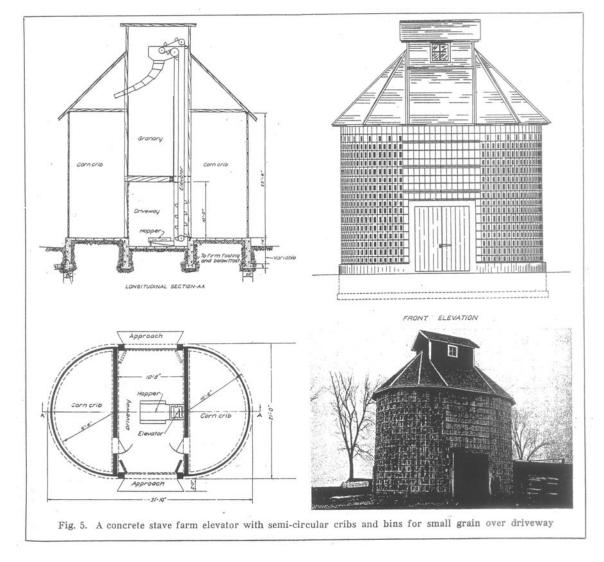
Combination corncrib-granaries could also be built of masonry. This oval, cement stave model contained two semi-circular corncribs, upper-level grain storage, and a built-in elevator. This illustration appeared in a 1921 article in *Agricultural Engineering* that indicated this style was common in Iowa. They were also built in southern Minnesota. From Kaiser and Foster (1921).
