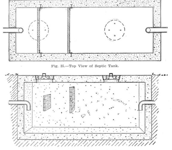
Fig. 36.-Lateral View of Septic Tank.
