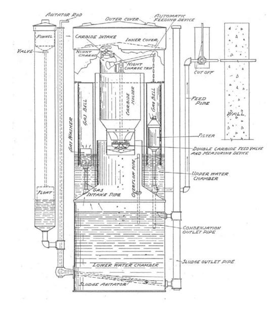
This acetylene or carbide gas plant was designed to be buried in a pit about 12' deep. The pit was usually located 50' to 100' from the farmhouse. Ground-level evidence of such a pit might include a circular pit cover, an agitator rod, and pipes, all located within an 8'-diameter circle. From Mowry's *Lighting Farm Buildings* (1915).
