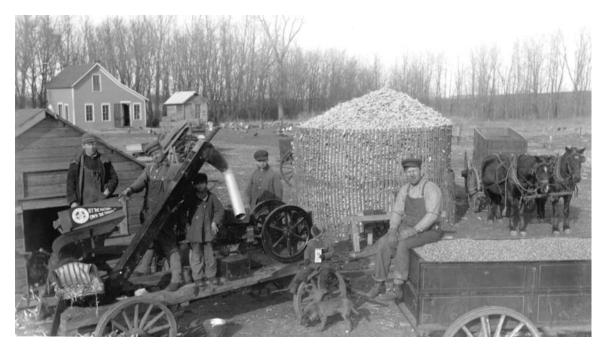
Farmers shelling corn using a sheller mounted on a flatbed. The shelled corn was placed in the wagon (right), and the ear corn into a simple corncrib (background) made of two rows of snow fencing. The two men on the left hold a banner that reads "Let the nation own the trusts," a socialist slogan. Location unknown, circa 1910. (MHS photo by Ole Mattiason Aarseth)
