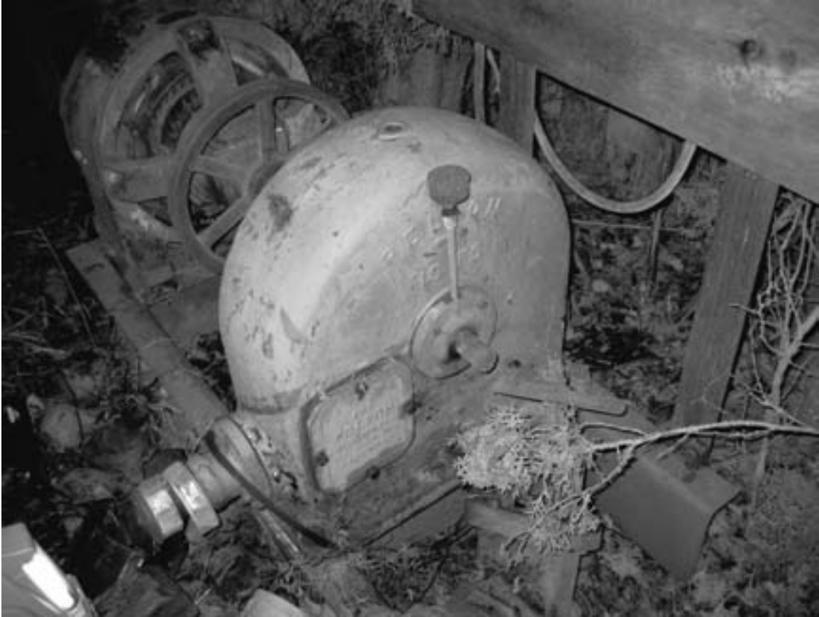
An 18"-diameter Pelton water wheel, used to generate electricity or power other farm jobs. Pelton wheels, made by Pelton Water Wheel Company of California, were recommended to Minnesota farmers by the University of Minnesota for generating electricity using the power of a farm stream. Photograph is from a web site called Rob's Pelton Place on the Net ( http://www.oldpelton.net/ ) 2005.
