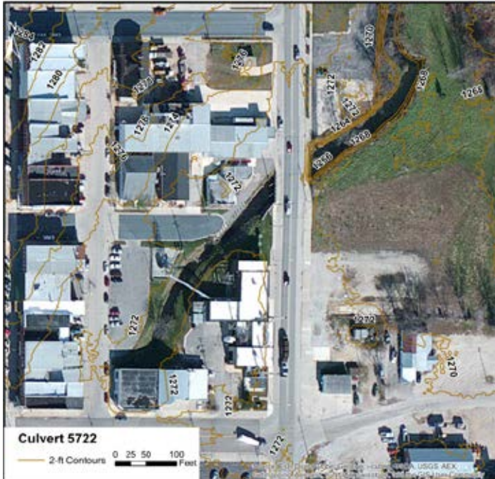
Figure 29: Plan View of Culvert 5722 Showing Elevation Contours
