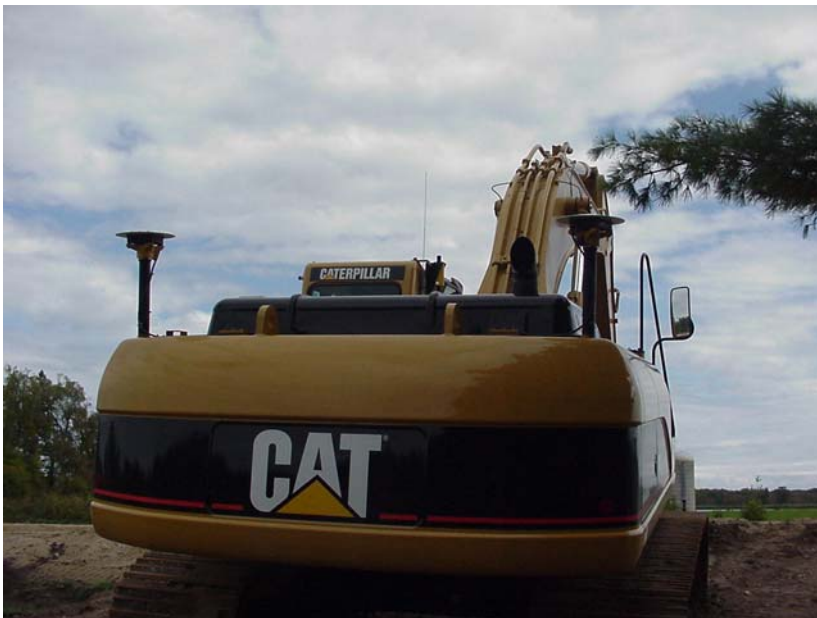
GPS on a Backhoe. Note the two Antennas
