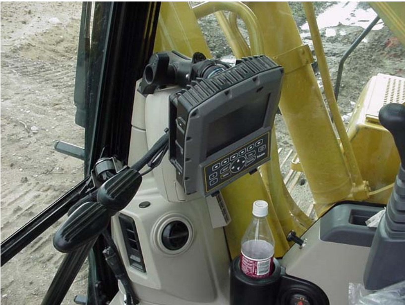
Operator's display for GPS inside of the Cab of a Backhoe.
