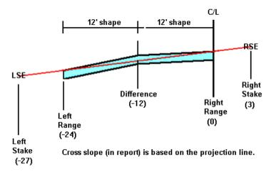
In this example the offset are in (\*) also we are using a 3 foot offset from the stake to the edge of the pavement.
