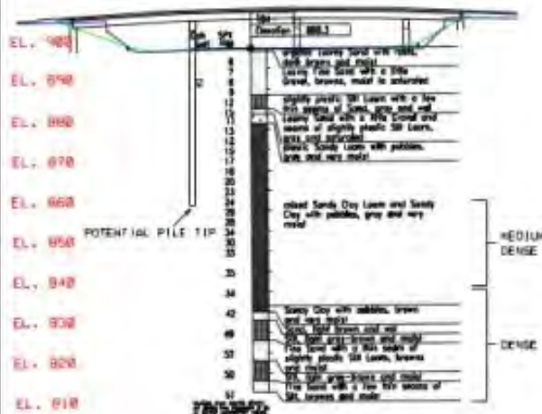
DENSE END BEARING LAYER WITH UPPER MEDIUM-DENSE LAYER
