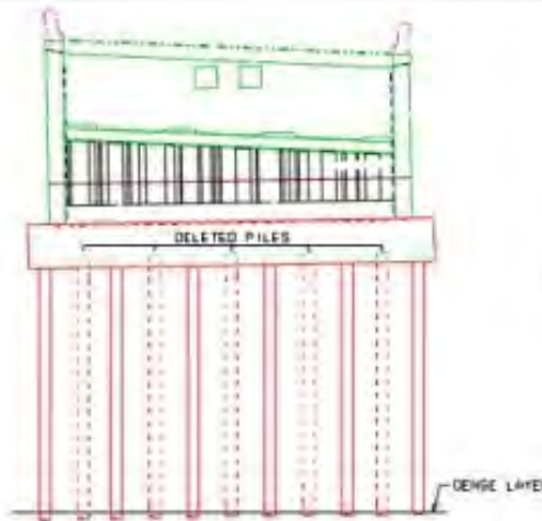
FEWER HIGH CAPACITY PILES WITH A RESISTANCE FACTOR OF 0.8
