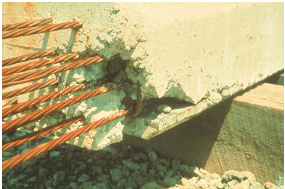
Figure 9.9.16 Spalling Due to Poor Concrete Placement
