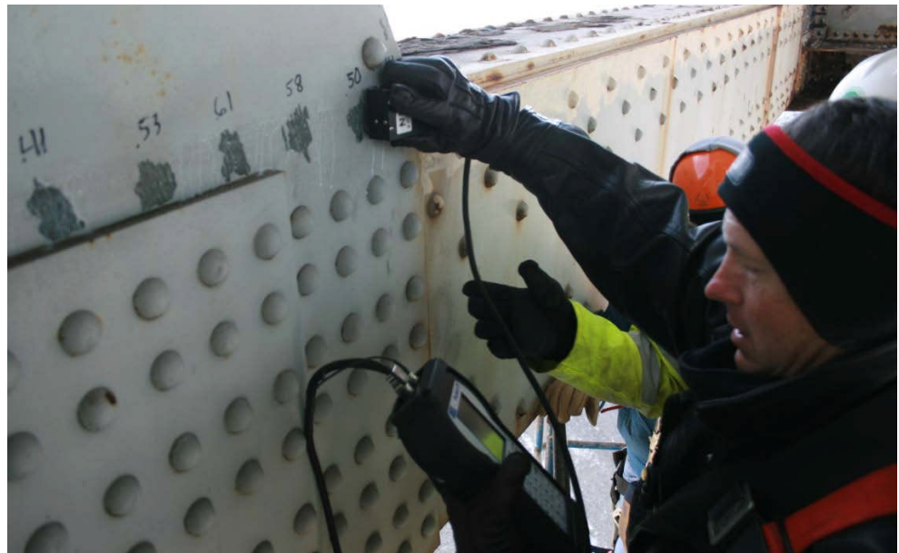
Figure 15.3.10 Ultrasonic Testing of a Gusset Plate Using a Phased Array
