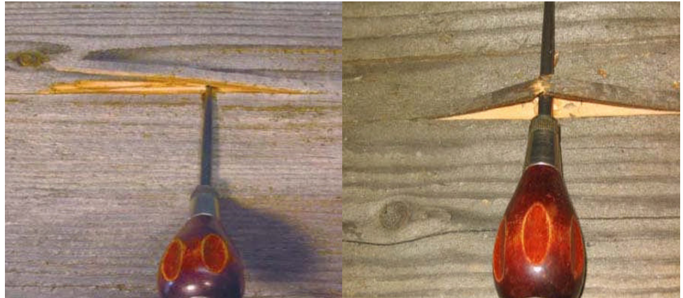
Figure 15.1.8 Pick Test: Sound Wood, Decayed Wood
