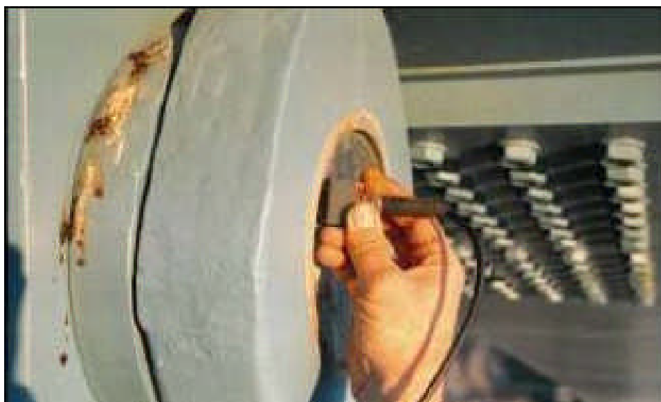
Figure 10.9.30 Ultrasonic Inspection of Eyebars Pin
