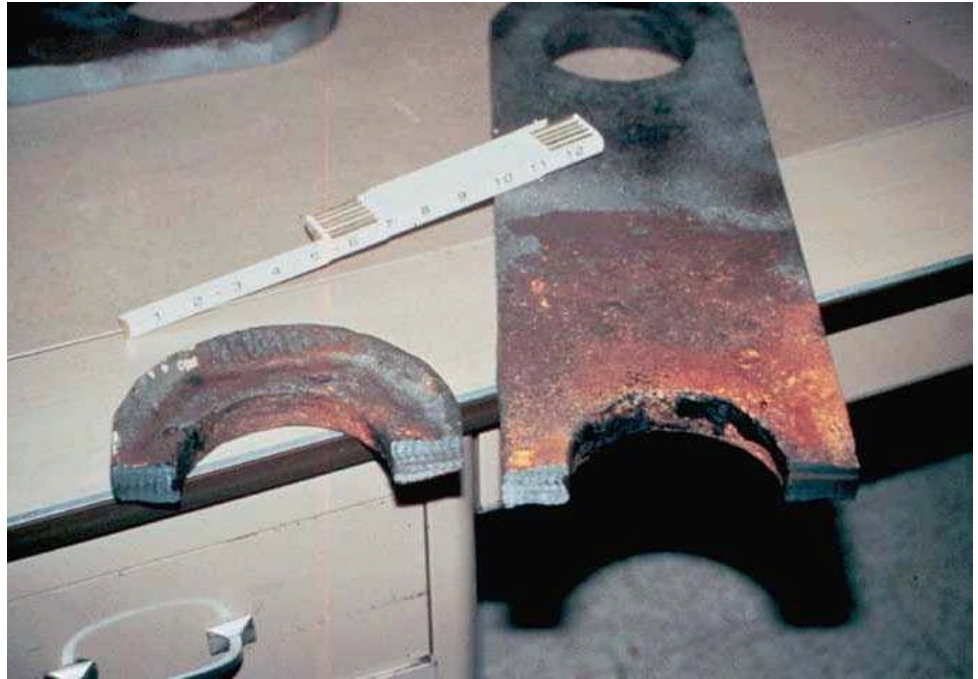
Figure 10.7.21 Corroded Hanger Plate
