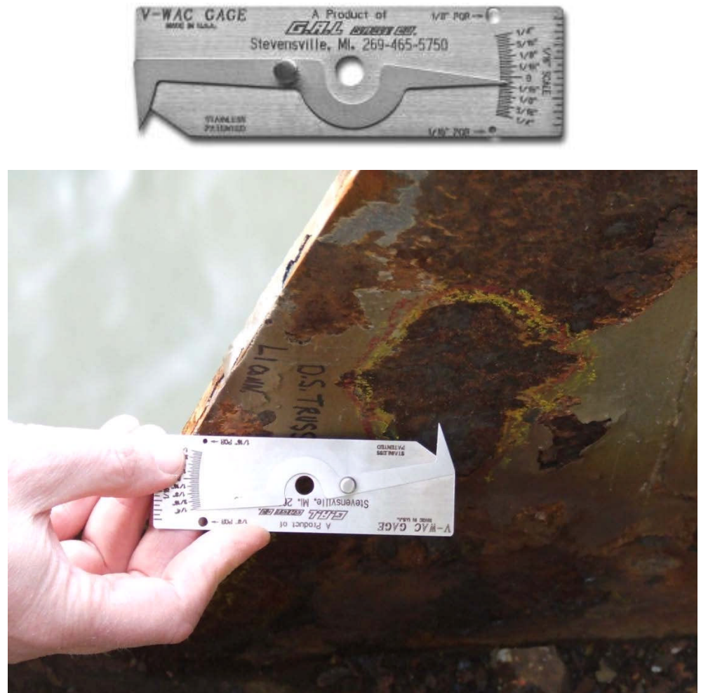
Figure 10.8.22 V-WAC Gage and Inspector Using the V-WAC in the Field to Measure the Section Loss of the Gusset Plate
