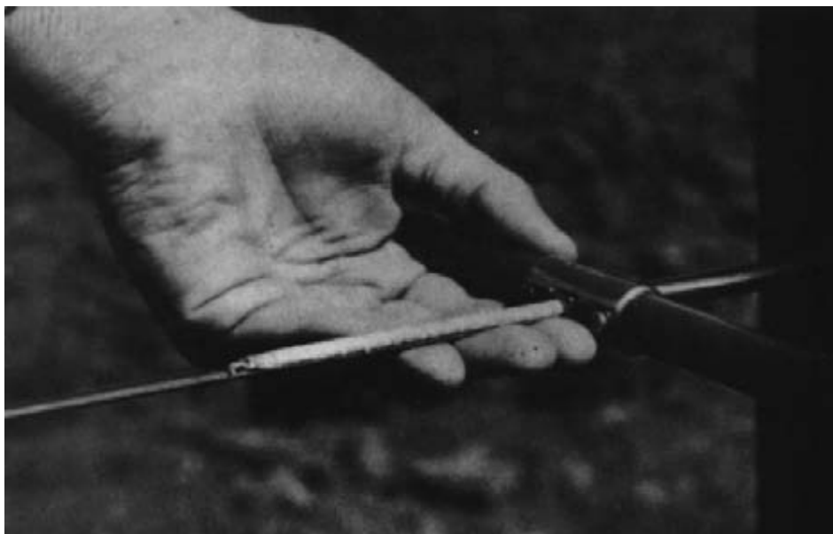
Figure 13-29. - Solid wood core removed with an increment borer. Such cores can be examined to determine the location and extent of decay.
