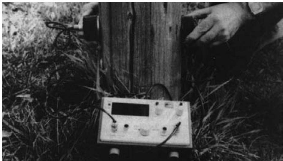
Figure 13-32. - A sonic inspection device for detecting internal defects in wood.
