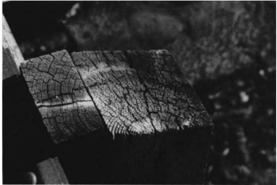
Figure 13-20. - Ultraviolet light degradation of the end grain of a guardrail post. Note the minor surface erosion of earlywood between the latewood (growth rings).
