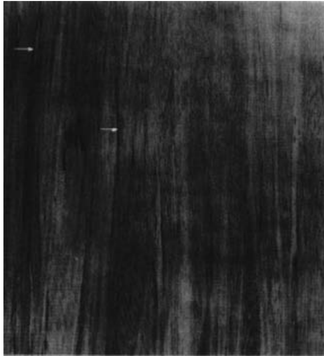
Figure 13-5. - Wood infected with white rot fungi. The decayed wood is abnormally light colored with dark streaks (arrows).
