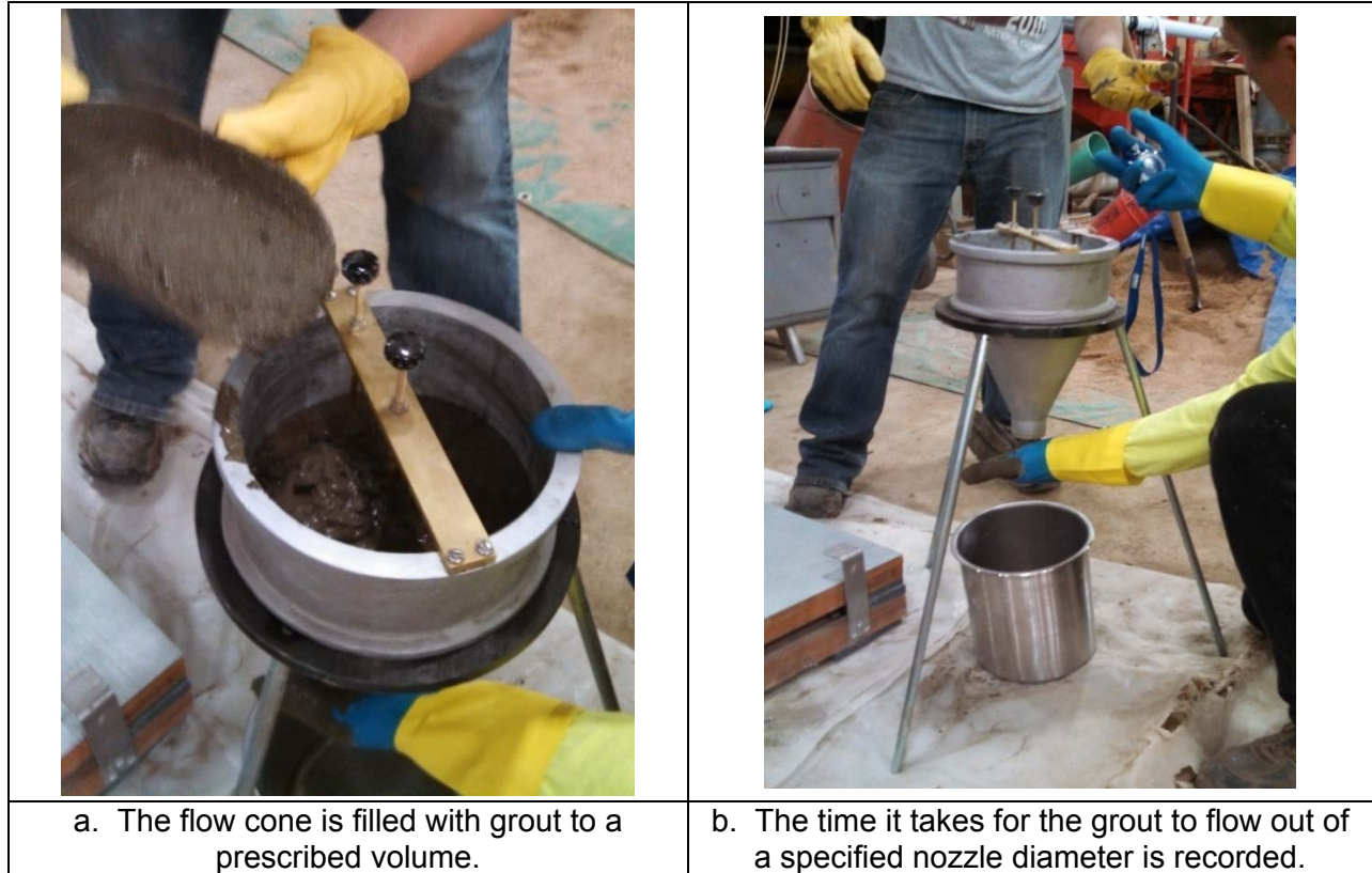
Figure 4.5. ASTM D6449, flow cone test device.
