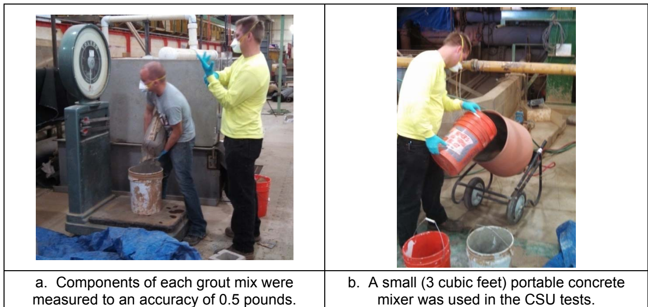
Figure 4.2. Grout mix tests at Colorado State University.
