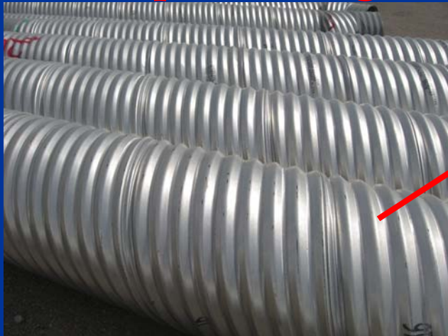
photo 0673 - aluminized Type 2 pipe - in spiral corrugation
