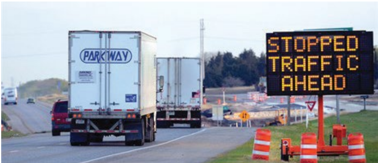
Figure 12 – Queue Warning System
