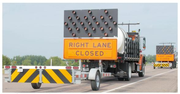
An ATMA truck follows the path of lead maintenance vehicles by useing connected and automated vehicle technology. The lead vehicle leaves "electronic bread crumbs" for the ATMA to follow, allowing the ATMA to operate autonomously. For this project demonstration, a safety driver will be in the ATMA vehicle at all times. In the future, ATMAs have the potential to increase safety during mobile work zone operations by not needing a driver, keeping workers out of harm's way.
