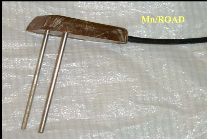
Time Domain Reflectometry Probe: Installed in all 40 test cells during construction. Manual measurement 1993-1998.
