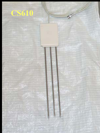
Time Domain Reflectometry Probe: Installed in reconstructed cells 27,28,33-35 (1999). Automated measurements 1999-present.
