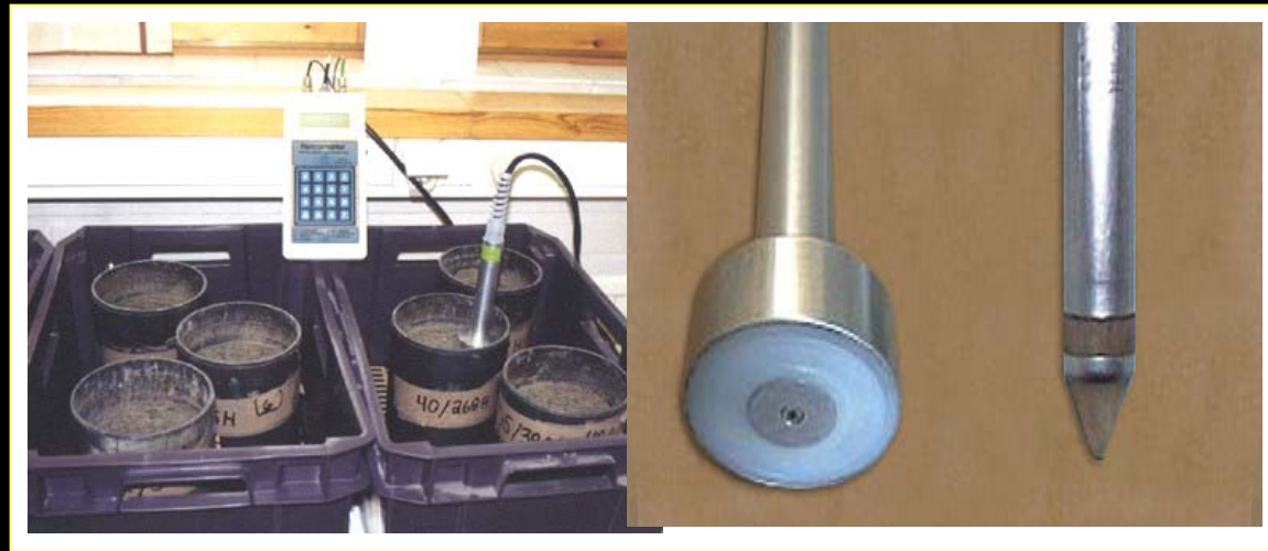
Water Content Reflectometer (uses tdr methods): Installed in reconstructed cells 27,28,33-35 (1999). Automated measurements 1999-present.
