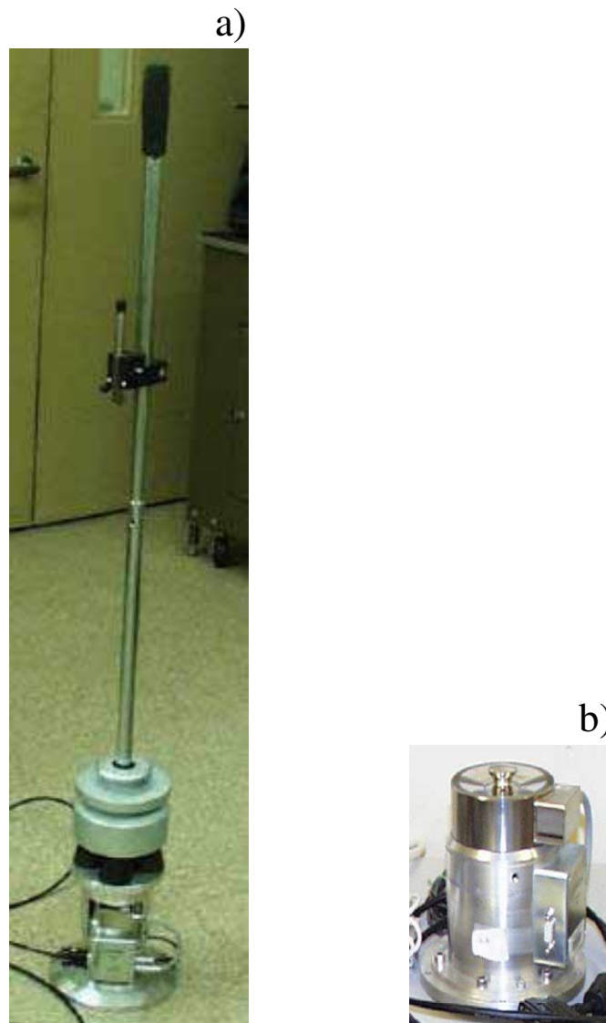
FIGURE 1 PRIMA 100 device: a) original configuration; b) modified configuration.
