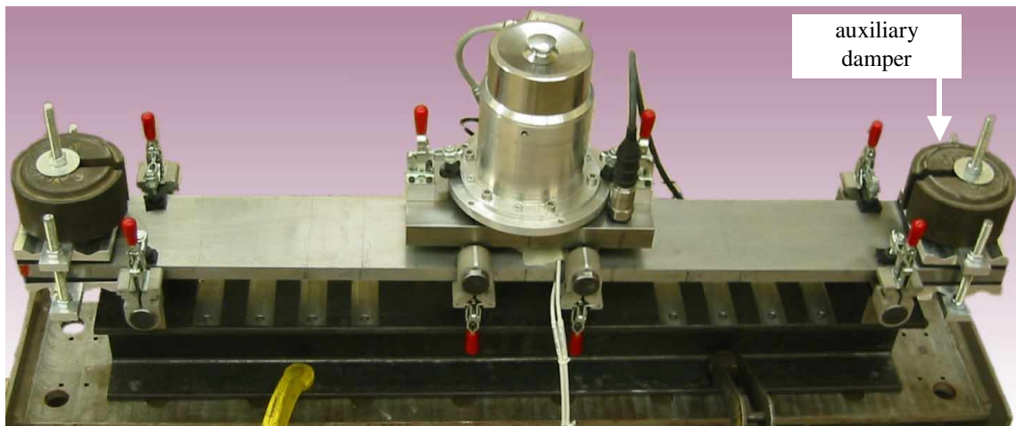
FIGURE 3 Beam Verification Tester (BVT): a) schematics; b) photograph.
