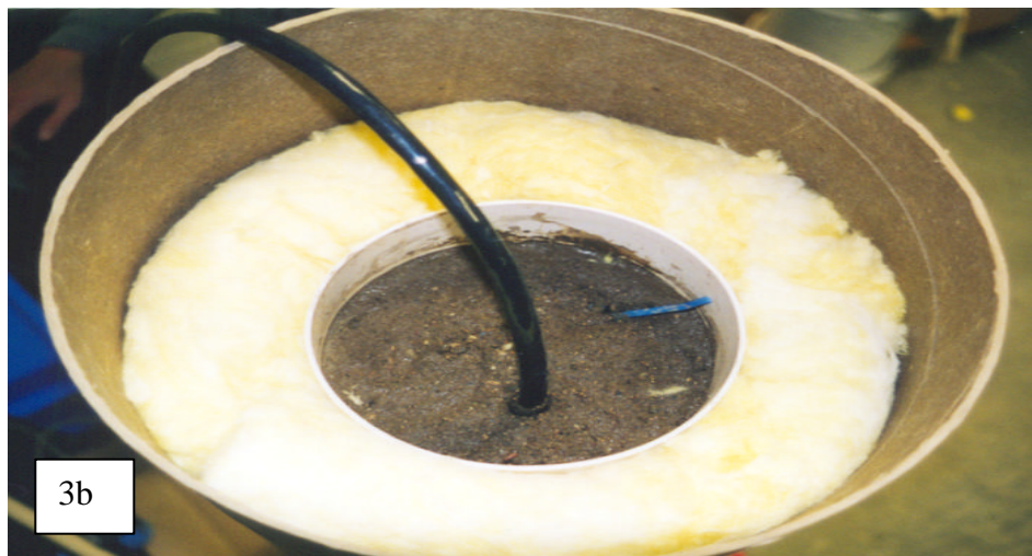
Figure 3 (a) Moisture Point probe and thermocouple installation. Two thermocouples were installed along the length of each segment. (b) R13 fiberglass insulation was packed between the soil column and the cardboard form. The insulation was used to confine the freezing to the surface of the soil column.
