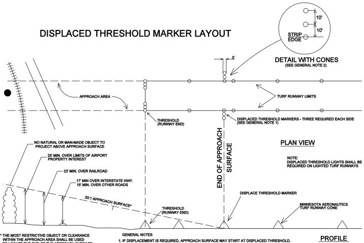
\* THE MOST RESTRICTIVE OBJECT OR CLEARANCE WITHIN THE APPROACH AREA SHALL BE USED TO LOCATE THE END OF THE APPROACH SURFACE FOR DISPLACED THRESHOLDS.
