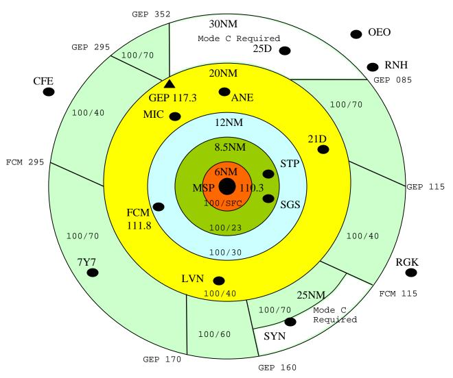
Transponder with Mode C is required for operation within 30 DME of I-MSP.
