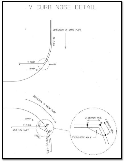
Figure 13: "V" Curb Nose Detail
