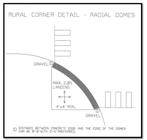
Figure 16: Flat Landing with Radial Domes
