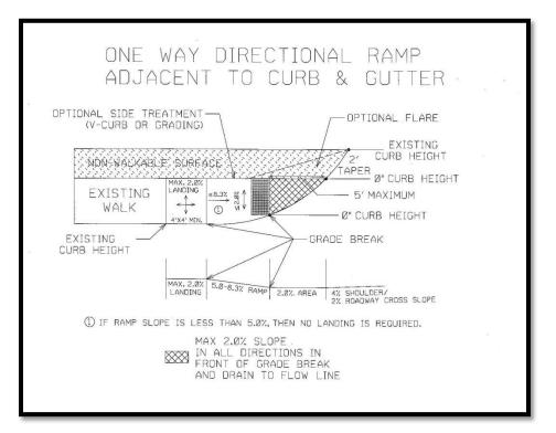
Figure 5: One Way Directional Ramp Adjacent to Curb and Gutter
