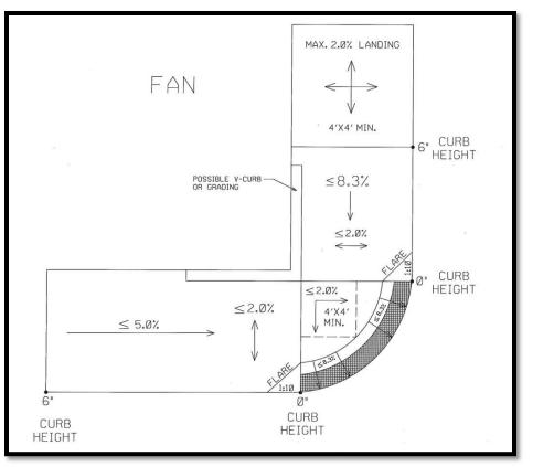
Figure 9: Fan Detail
