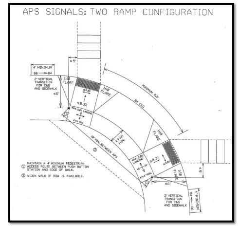
Figure 14: Accessible Pedestrian Signal
