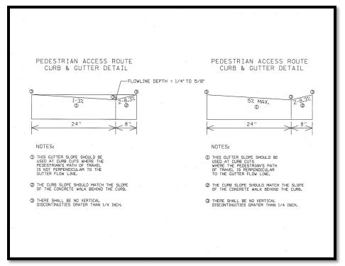
Figure 12: Curb and Gutter – Standard and Pedestrian Access Route
