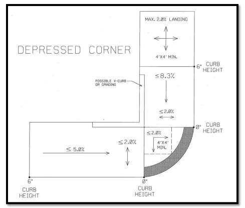
Figure 8: Depressed Corner Detail
