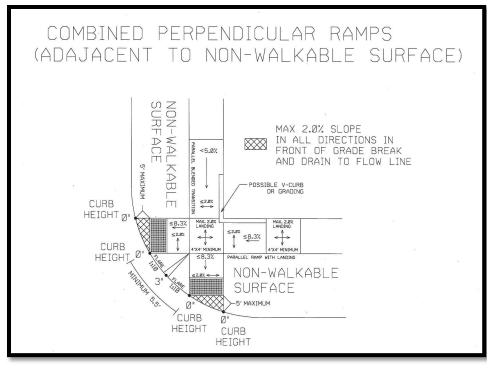
Figure 4: Combined Perpendicular Ramps Adjacent to Non-Walkable Surface
