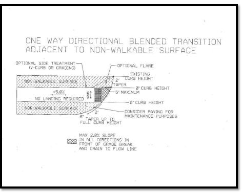
Figure 6: One Way Directional Ramp Adjacent to Non-Walkable Surface
